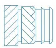
Has been developed for installation into thermoplastics where the design incorporates a tapered hole configuration. The parallel body design combined with the opposing helical knurl bands enables users to achieve up to a 25% increase in productivity by the ability to reduce the recommended dwell time compared with standard tapered hole inserts.
