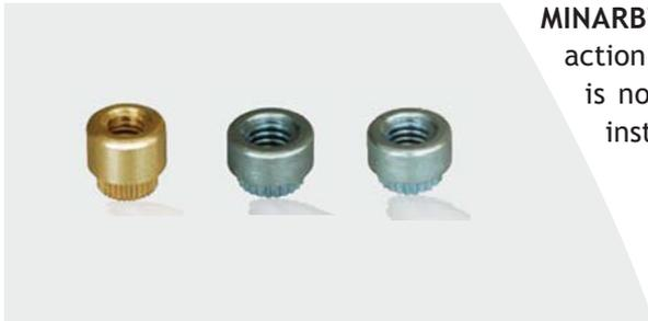
MINARB<sup>®</sup> can be installed using both an “impact” and a “squeeze” action, allowing both hand and machine installation. Sheet hardness is not critical as the bush deforms rather than the sheet, during installation.
