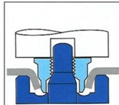
Force is applied to the nut/stud which enables it to plunge the material
