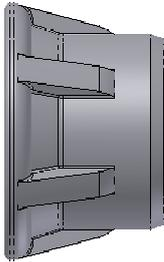
Flangeform Clinch Nuts are threaded fasteners with unique ribs designed for installation into thin gauge materials. The fastener plunges the pre-punched hole and wraps itself around the material whilst the ribs embed themselves providing an integral high strength attachment point.
