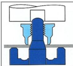
Material is placed over the mini-die and radially located on the pin
