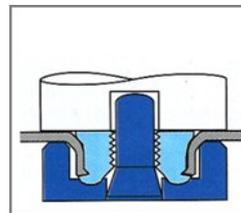
The nut/stud is formed around the parent material by the profile of the mini-die.
