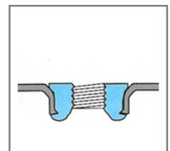
The nut is flush and integral with the component
